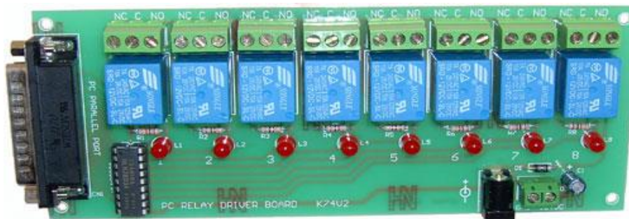
Figure 3. Relay control board
